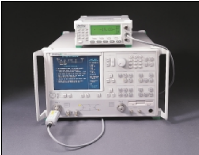
Use a power meter for a flat test port power correction.
