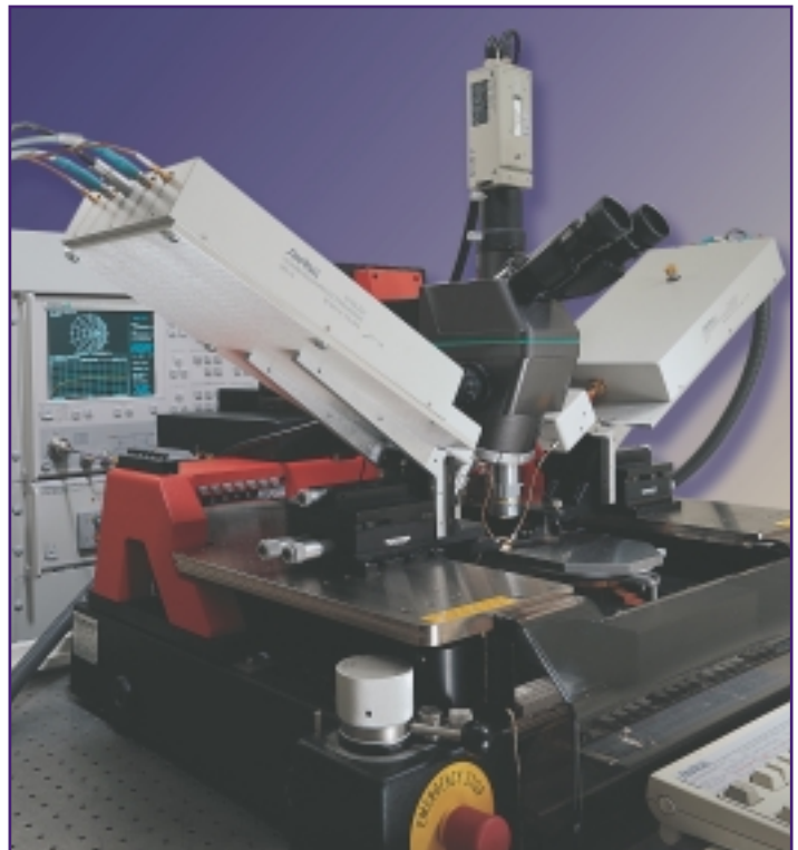
Complete on-wafer measurement solution: ME7808A integrated with Karl Suss PA200 probe system
